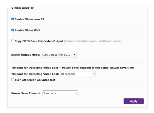
Scaler Output Mode: This feature is used to set the output resolution from the UHD60 Decoder. Default is to use resolution specified by the display EDID. "Auto Detect (Per EDID)".
