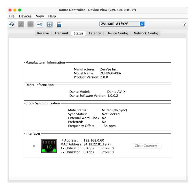
Some ZyPerUHD60 Encoders and Decoders support Dante AV-A. This means every endpoint can be configured to support both Dante transmission and receive functionality.
