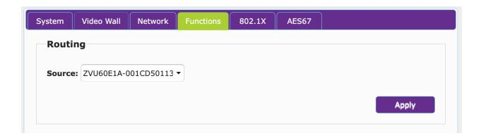
If you click on the small down arrow in this Source box you will bring up a listing of all available encoders on the network. Selecting a different encoder will cause all video/audio/USB etc.. signals to switch to this new encoder.
