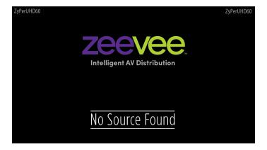
The default background can be changed from the ZyPer Management Platform GUI in the **Display Grid** page **Config** tab.
