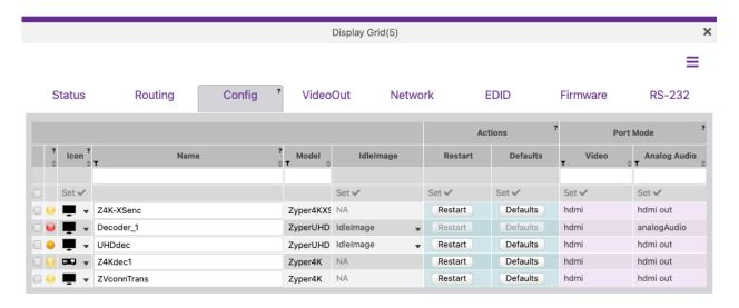
For the desired decoder, select the "**IdleImage**" option. Here you can upload a new background. The uploaded file must meet these requirements.
