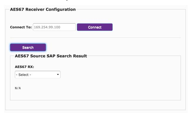
Here you can search for any AES67 streams available on the network. Note that any streams must have appropriate SAP to be discovered by the UHD60 Decoder.
