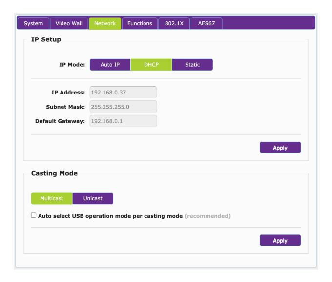
Always be careful when assigning Static addresses to units. It is important to never duplicate a Static address.
