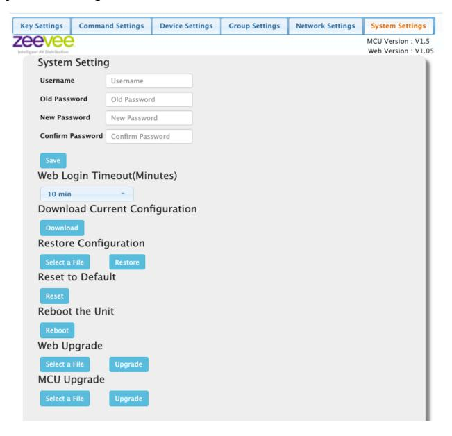
The System Settings tab allows to perform such functions as settings a new admin password, selecting preferred language, settings a web UI timeout, save the current configuration to a binary file, restore a saved configuration, reset the unit to factory defaults, reboot the unit and perform web UI and MCU upgrades.
