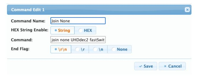
The example above with the name "Join None" is for the API command "join none UHDdec2 fastSwitched"
