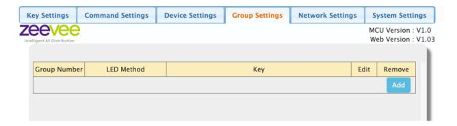
Group Settings is available to group the buttons according to the relationship and functions of commands configured to the buttons. Basically controls how the buttons light up when pressed.
