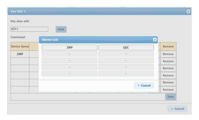
This will bring up the Command Destination box to allow you to select any of the commands you previously created be used when the button is pushed.
