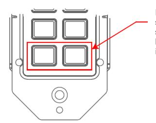
Press and hold the 2 bottom buttons simultaneously and hold for about 8 seconds. This will cause all 10 buttons to blink 3 times and indicate the ZyPerPad is being reset to factory defaults.
