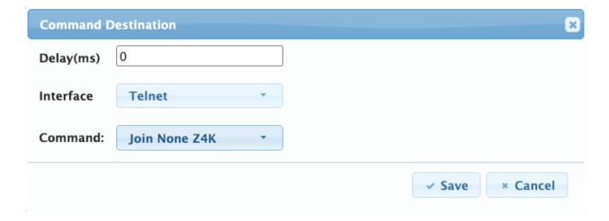
Set **Delay** to 0ms, Set **Interface** to Telnet or RS232. Click the box next to **Command** and select any of your preconfigured commands.
