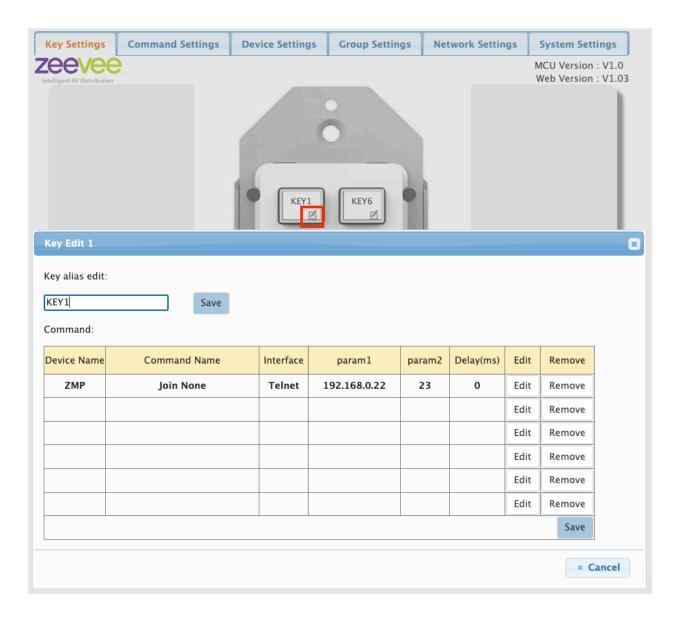
Click on the bottom right corner of the desired button. Red box in image above for Key1.
