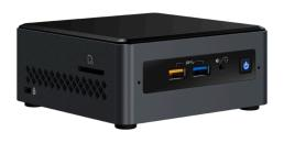
All installations will require a ZyPer Management Platform (ZMP). This device controls the operation and manages the connectivity between endpoints. The management platform is a hardened controller node that must reside on the same logical network as the ZyPerHD Encoders and Decoders. It runs a ZeeVee application as its sole function. The application presents an API to potential third party management platforms as well as hosting its own management application.
