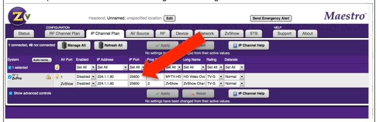
**STEP3:** Enable the IP stream function and APPLY the changes. Note that Maestro does not effect the changes indicated on a form until the APPLY button is hit.
