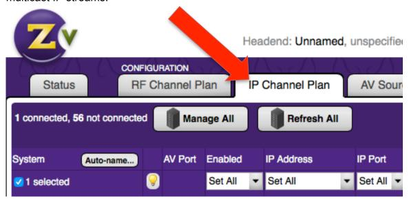
Navigate to the IP Channel Plan page in Maestro for the ZeeVee product being controlled. In this case it is a ZvPro810i-NA
