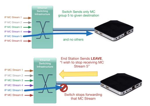
So by virtue of the fact that the switches are intelligent enough to only forward the multicast groups of interest, there is no limit on the number of offered streams (channels) that can be carried. No link should ever be swamped.
