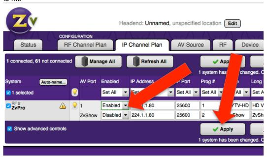
At his point the ZeeVee encoder/modulator will be sending the specified IP stream to its Ethernet interface.
