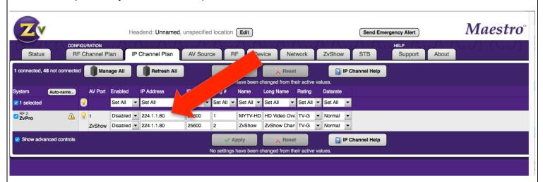
Each unique ZeeVee encoder/modulator IP stream on the Ethernet network should have a unique multicast address.
